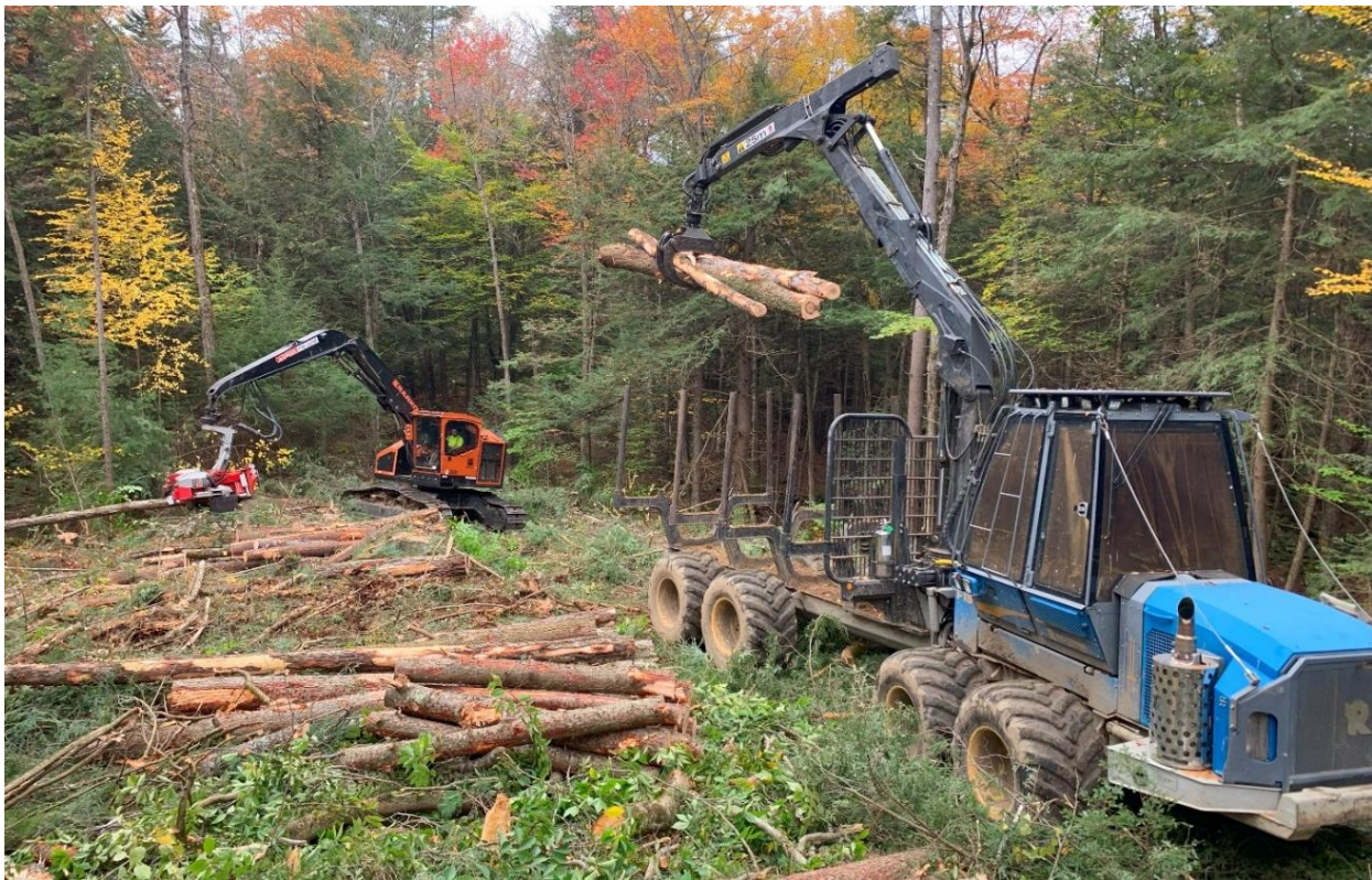
One of Long views crews at work with a Barko 260 harvester and Rottne F15 forwarder
