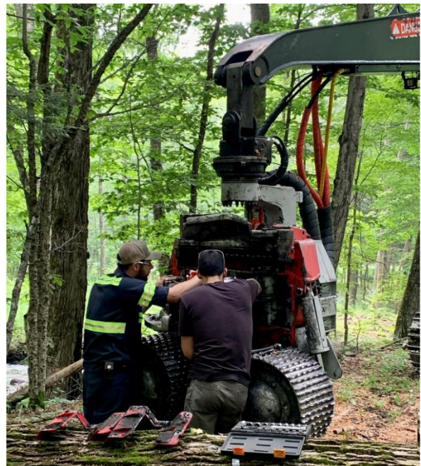
Mechanic and operator working on a Log Max 7000XT processing head
