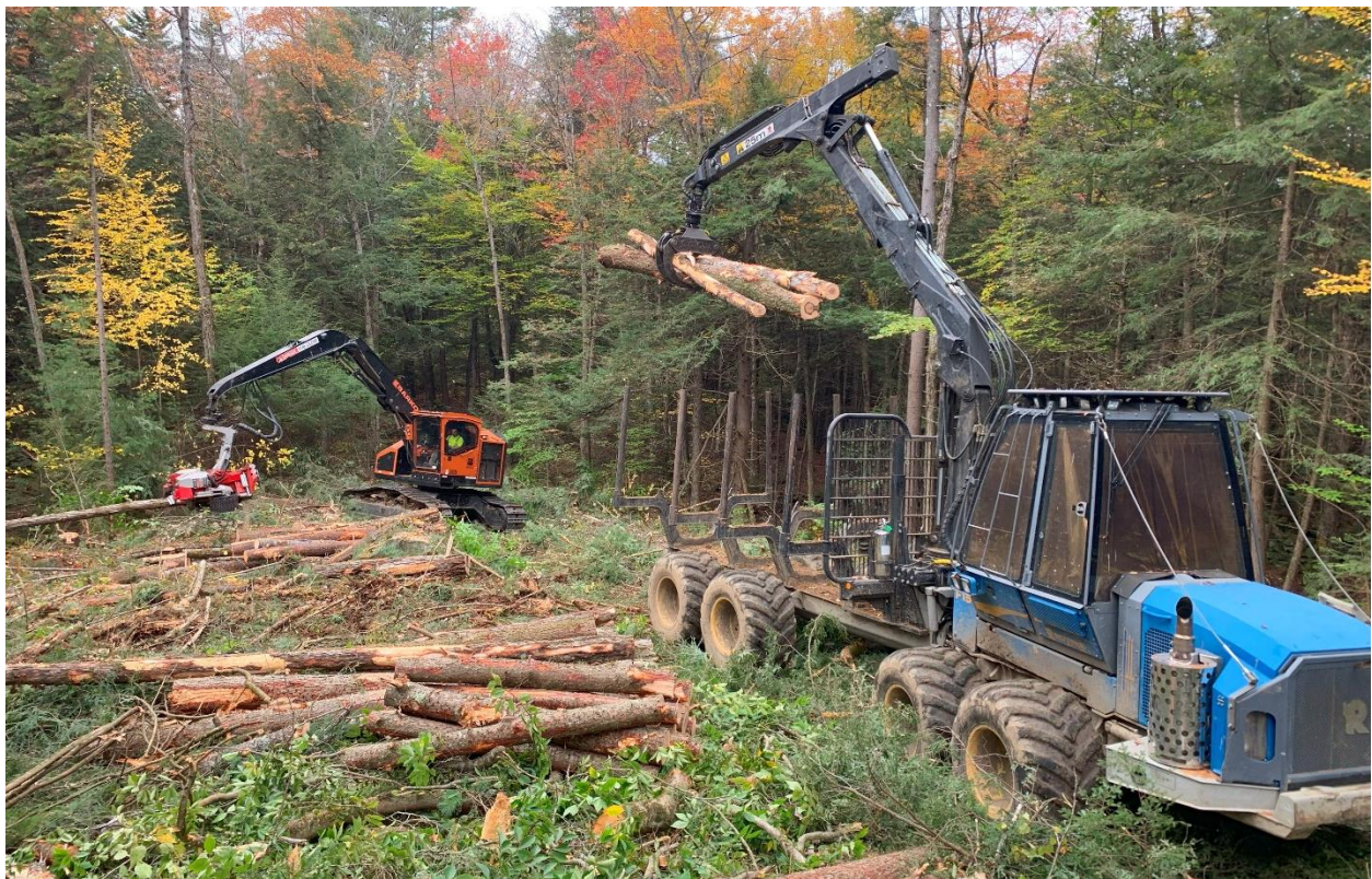
One of Long View's Barko 260 harvesters at work with a Rottne F15 forwarder
