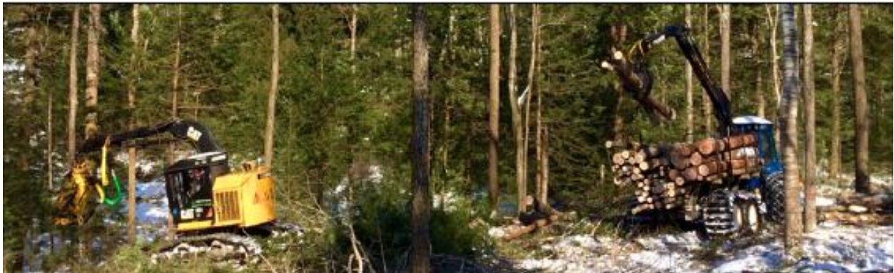
One of Long View's harvester and forwarder teams doing thinning work in the forest.
